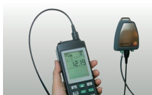
Inspection of transmitters with 4 to 20 mA interface
