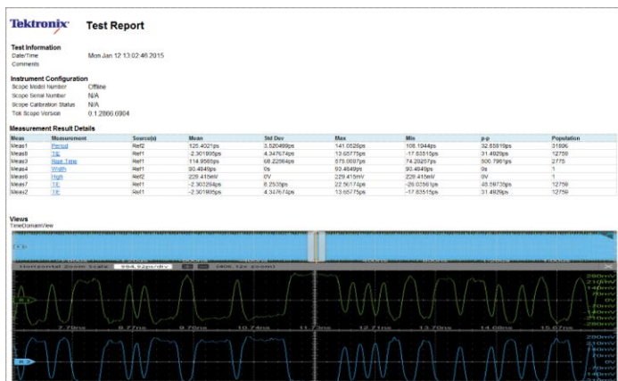
Complete test report includes setup details, measurement configuration and results, and plots
