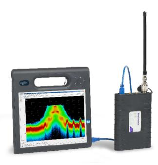
signal. In general most spectrum analyzers provide the same display; they show lower frequency signals on the left hand side of the display and higher frequency signals on the right hand side of the display. The three basic controls for most spectrum analyzers are; Frequency, Span & Amplitude (Reference Level). With these three controls we can control the view of the spectrum. The next question is "what am I looking at"?
