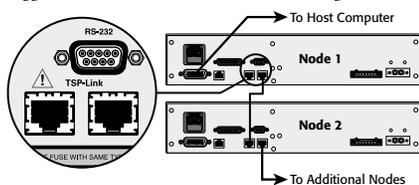
Each Model 2651A has two TSP-Link connectors to make it easier to connect instruments together in sequence.
