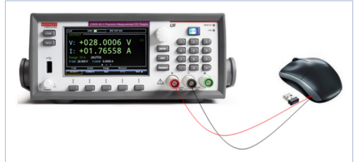
Figure 8. 2280S is connected to the DUT
