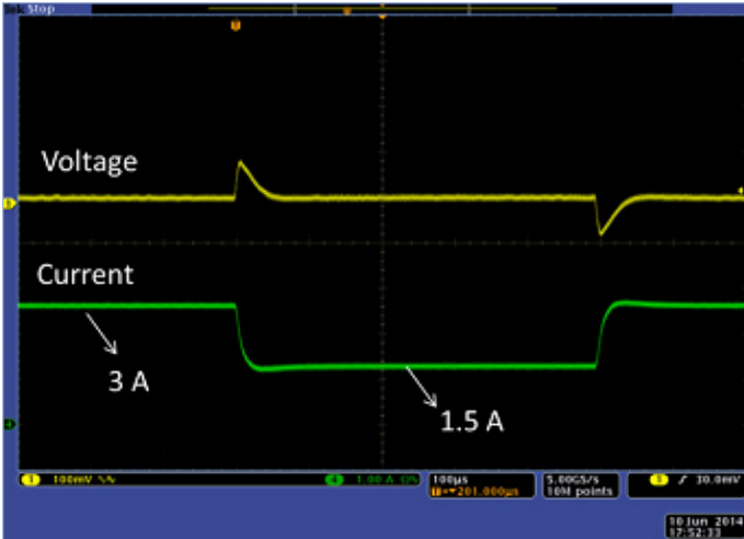
Figure 7. The load current instantaneously transitions from 3 A to 1.5 A and then back to 3A. The output voltage recovers within a very fast, 38 us
