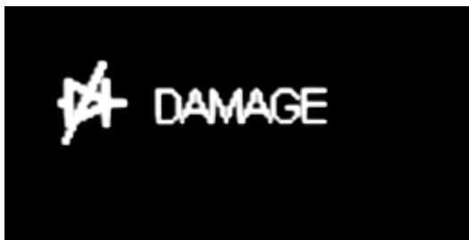
Figure 3-14: Display of Diode Measurement (Damaged Diode)
