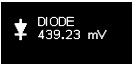
Figure 3-13: Display of Diode Measurement (Good Diode)
