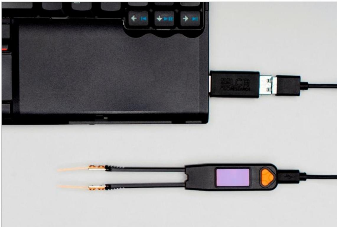
Figure 3-1: Connect LCR Pro1 to PC
