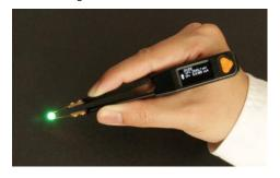
LCR Pro1 Plus offers an additional LED testing function. In LED testing, it lights up the LED and displays its electrical parameters, such as polarity, voltage and current. When testing bi-directional LEDs, the electrical parameters will be displayed in each direction.
