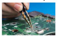
The redesigned gold-plated tips are more precise than ever. You can use them to pick up and measure SMD components quickly and reliably, even for the most tiny parts with 01005 size.
