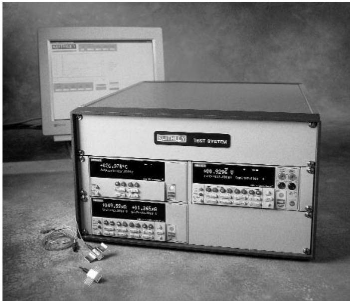
Rack Mounted L-I-V System
