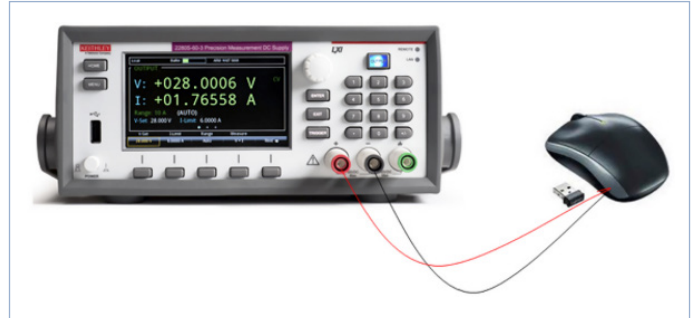
Figure 8. 2280S is connected to the DUT
