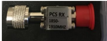
Interference Mitigation Filter Tuned to pass low level PIM signals Reject Tones from the iPA, and any other high power signal at the sites
