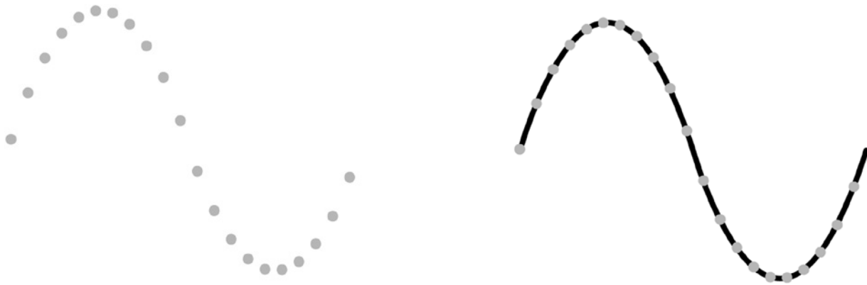
Figure 17. (Left) A series of sampled points representing a sine wave; (Right) the reconstructed sine wave.
