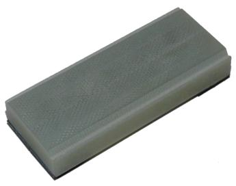
Using the M321 is very intuitive: place a few DUT's in the top surface and gently push them over one edge of the fixture. One edge is for micro chips and the other is for larger chips. The DUTs will slide down to the bottom of the angled groove—if the DUT lands on an end, simply push it over so it is laying on a side and the ends are presented for testing as shown in the photo below.
