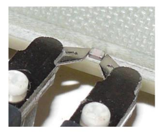
Use the smaller groove for micro chips, for example 01005 (metric 0402) and 0201 (metric 0603). Use the large groove for larger chips.
