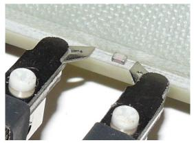
Close the tweezers so they grip the DUT, making sure to use the fixture surface to guide the tweezers electrodes so the grip angle is maintained. Pick up the chip and record the test results.
