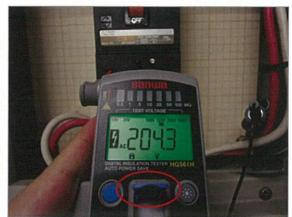
■When the circuit to be measured is in a hot-line condition(≥ 30 V ac/dc ), and under this condition, even if the TEST button gets pressed, the instrument will not generate any test voltage. Turn off the circuit to be measured, and then measure again.
