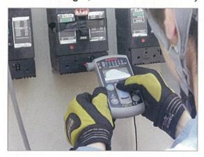
▲ Measuring the value from the top of the terminal cover with HG561H
