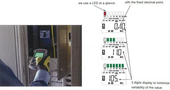
▲The LED light embedded in the leading end of the main unit and the back light of the liquid crystal display illuminate at the same time, and the lighting lamp illuminates a place to be measured, and the LCD has a backlight.
