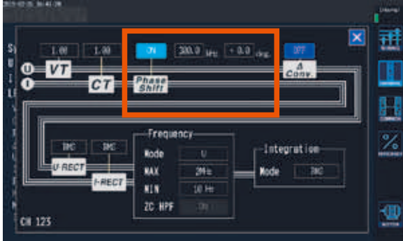
Enter phase calibration values for each frequency to correct high-frequency phase characteristics.
