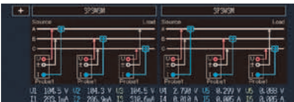
Wiring confirmation function, to avoid wiring mistakes
