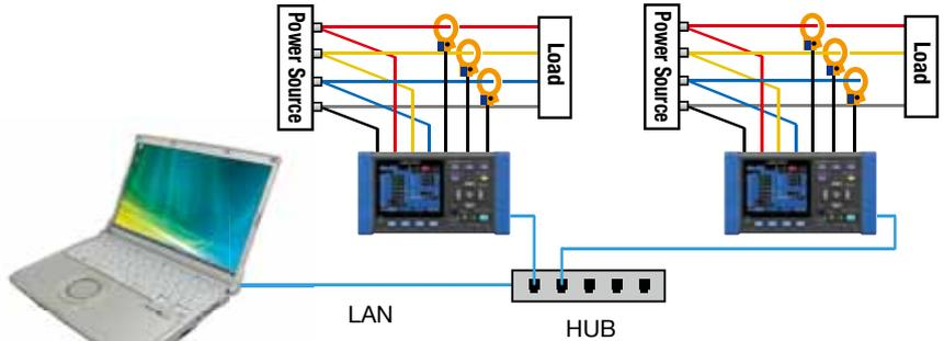
Files recorded in the PW3360-20 internal memory or SD card are accessible by LAN or USB connection, and are downloadable using the free **PW3360 Setup and Download Software**.
