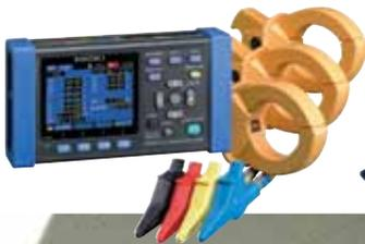
Record power consumption on an SD Card\* at specific intervals. Load the data into the PC.
