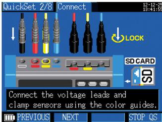
Make proper connections simply by observing the colors of the displayed leads.
