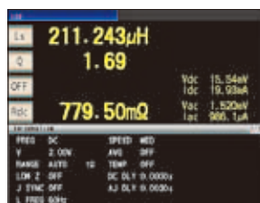
L, Q and Rdc continuous measurement screen
