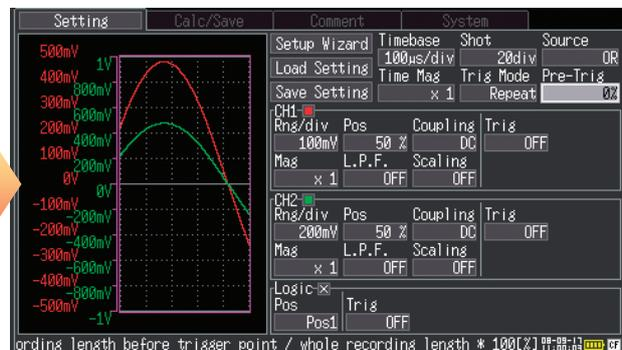
When powered on, the Settings screen appears along with the waveform monitor, and the new Setup Wizard blinks. By activating the Setup Wizard, you can easily navigate by following the simple instructions. Soon you will be operating the device like a seasoned professional.
