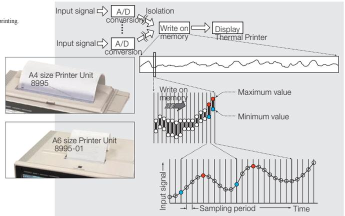
Because of this, the volume of recorded data is compressed while following steep fluctuations of the measured input voltage.
